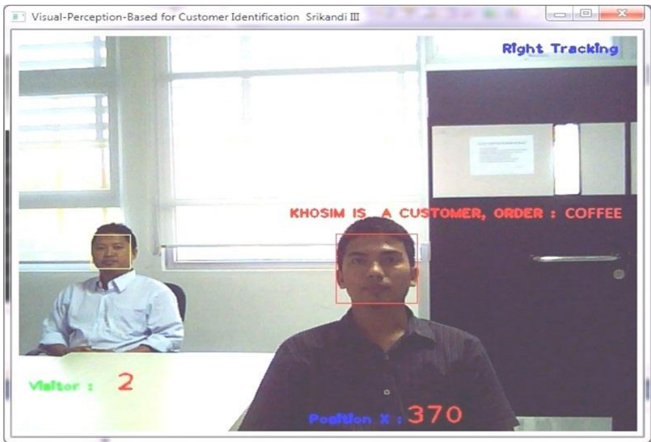
Figure 11.7 An example of face detected and recognized together with his order using our framework of face recognition system.
