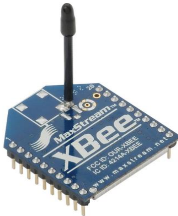
Figure 4.5 Wireless communication using XBee.
