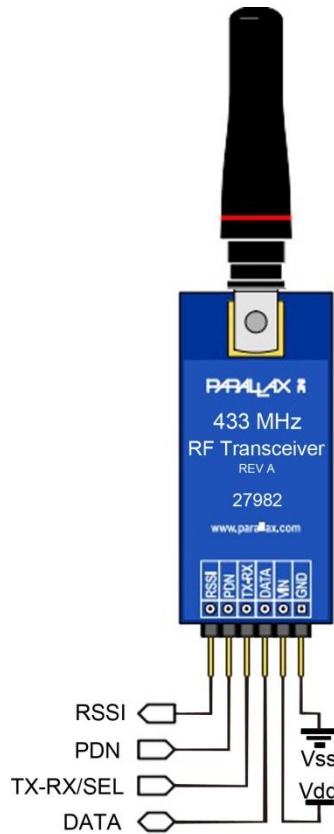
Figure 4.4 Wireless communication using 433 MHz Transceiver.
